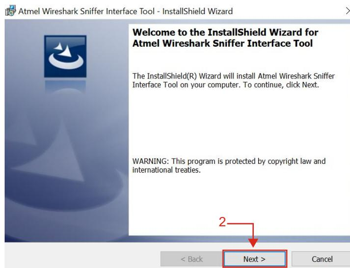
3. Install the Wireshark Sniffer Interface Tool in the default location, `C:\Program Files (x86)\Atmel\Atmel Wireshark Sniffer Interface Tool\Atmel Wireshark Sniffer Firmware`.
