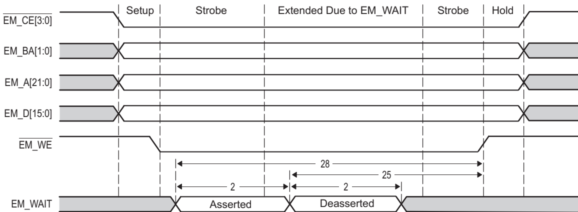
图 11-55. EMIF16 EM_WAIT Write Timing Diagram
