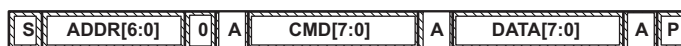
Figure 7. Attempt to Write a Read-Only Address (Nack After Data Sent By Master)
