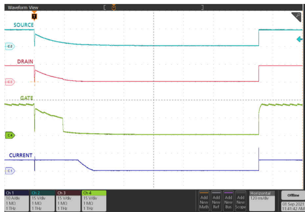
图 9-4. Response to ISO 7637-2 Pulse 1
