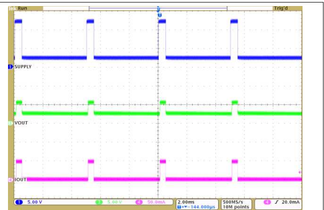
Ch. 1 = V_{(SUPPLY)} Ch. 3 = V_{(OUT)} Ch. 4 = I_{(OUT)} f_{(PWM)} = 200\text{ Hz} Duty-cycle = 10% SUPPLY dimming between 2.5 V and 12 V
